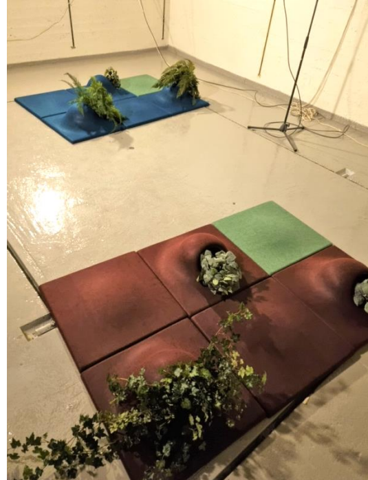
Figure 5: A mix of three PlantPanels and three PlainPanels absorbers 580 x 580 mm, measured for sound absorption area.
