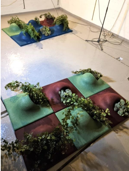
Figure 4: Two groups of six PlantPanel absorbers with artificial plant 580 x 580 mm, measured for sound absorption area.
